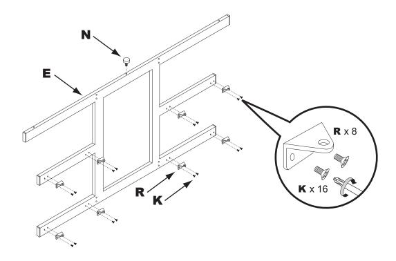
1-Fasten glass supporter (R) to the frame (E) with screws (K). Fasten glass protector (N) to the frames (E).
